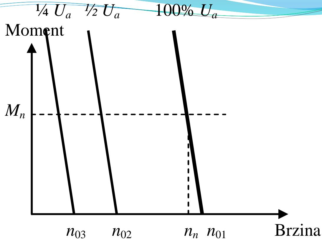
$$\omega_m = \frac{U_a - R_a \frac{M_m}{K_m}}{K_e} = \frac{U_a}{K_e} - \frac{R_a}{K_e K_m} M_m$$
