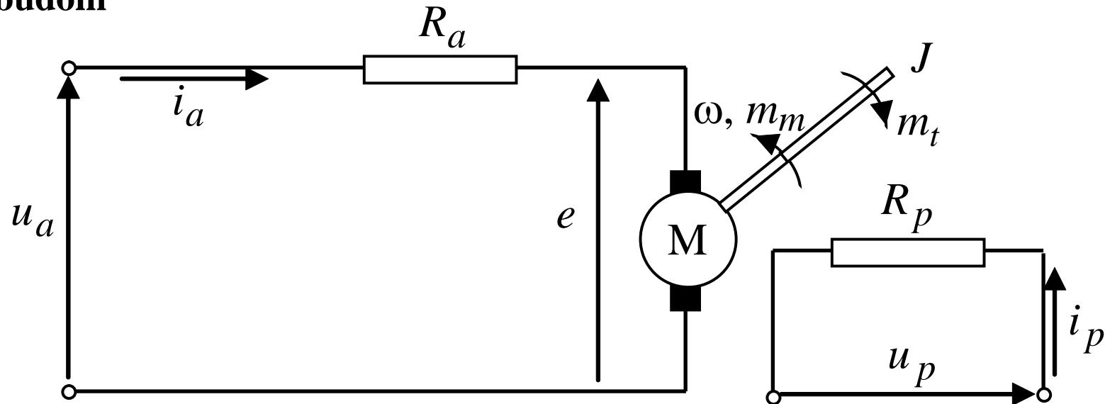
$$1 \dots U_a = R_a I_a + \Phi \omega$$
